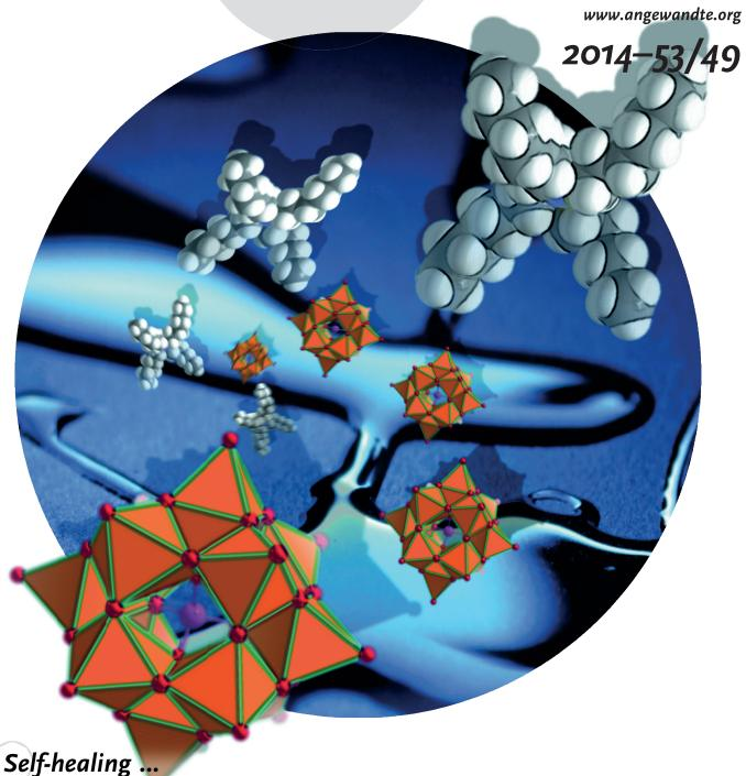
... corrosion protection is provided by functional polyoxometalate ionic liquids (POM-ILs) coated onto metal surfaces. In their Communication on page 13596 ff., C. Streb et al. utilize POM-ILs, which are hydrophobic, acid-resistant, and form mechanically stable films, to protect copper metal against acid corrosion. Mechanical damage to the coating is self-repaired in less than one minute through the unique rheological properties of the compounds.
